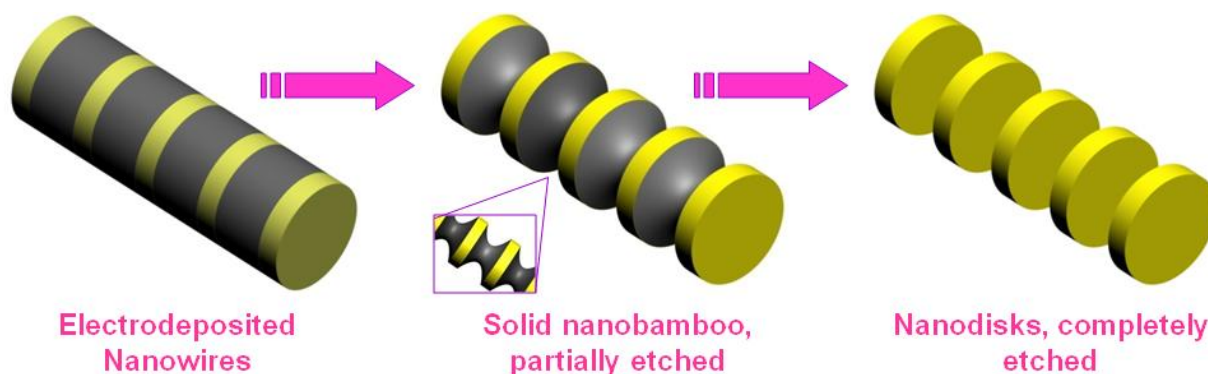
Figure 4-32 Schematic illustration of the procedure for fabrication of porous nanobamboo and nanodisks through selective electrochemical etching of Au/CoAu nanowires
