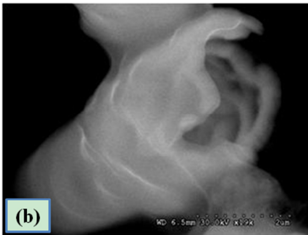
Figure 4-61 SEM images of Au 25 nm / CoAu 150 nm nanotubes with diameter of 2.0 μm taken (a) before and (b) after electrochemical etching for 900 s
