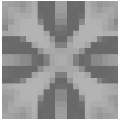
Fig. 4. Stress constrained design for maximum torsional rigidity.
