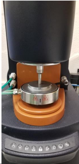
Figure 4 . TA Discovery HR-2 rheometer used for experiments.
