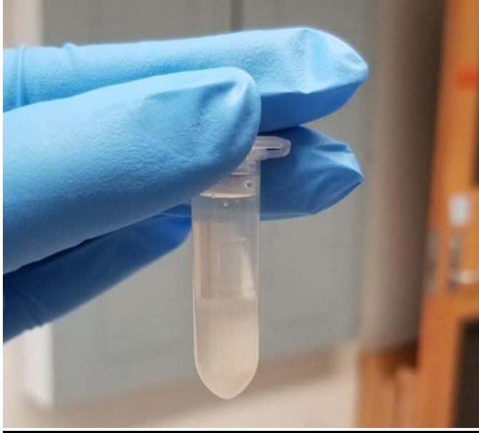
Image 3. Alligator gelatin with mTG after mixing with vortexer, heated at 60 °C for 30 min, and rested for 5 minutes at 37°C.
