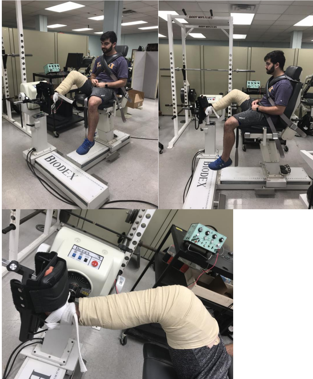
Figure 5. Biodesx Systems III Dynamometer set-up and positioning for ankle and knee joints with electrical stimulation.
