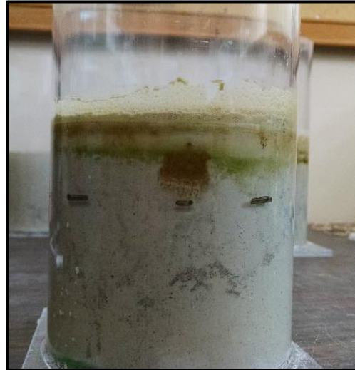
Figure 2: Photograph of jar for sedimentation rate 3 after 11 weeks of sedimentation with biofilm. Black dashes indicate the top layer (0-3 cm) to extracted for sampling and analysis.
