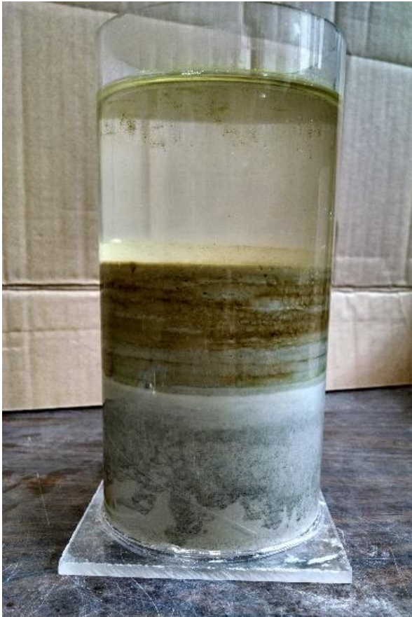
Figure 1: Photograph of jar for sedimentation rate 5 after 11 weeks of sedimentation with biofilm.
