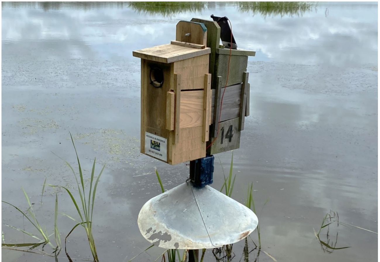
Fig. 2. Duplex-style nest box consisting of one new (left) and one old (right) nest box on a singular pole with a conical baffle. The waterproof container housing electrical components is zip-tied below the nest boxes, while the solar panel is fastened to the top of a nest box with wood screws facing southward. The loop-style antennas are zip-tied around the nest box entrance through four drilled holes, with antenna 1 affixed to the new nest box and antenna 2 affixed to the old nest box.
