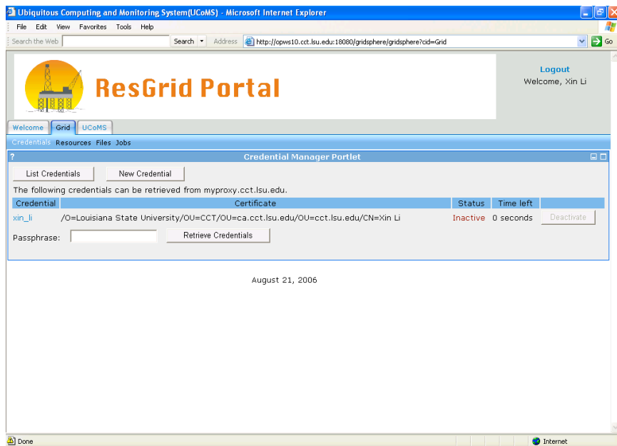
(b) Grid security. A Grid Security Infrastructure certificate is retrieved from a proxy to provide user authentication to access Grid resources.
