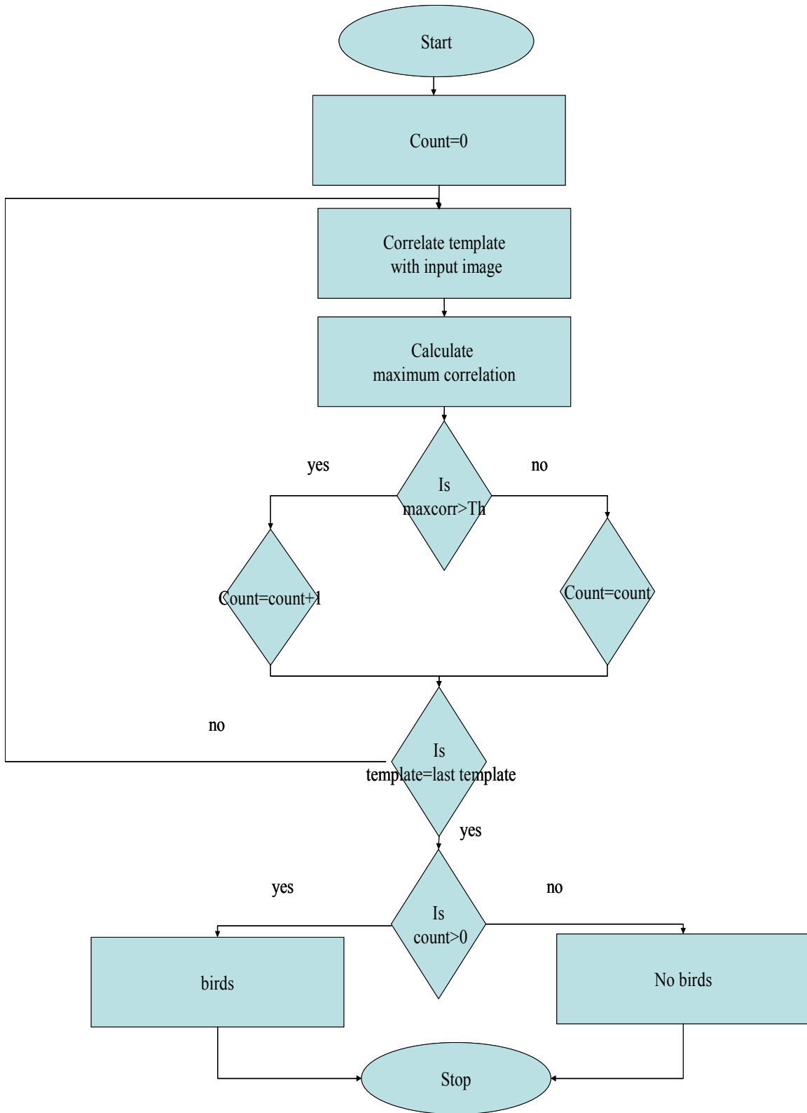
Fig: 3.11. Flow chart explaining the template matching technique
