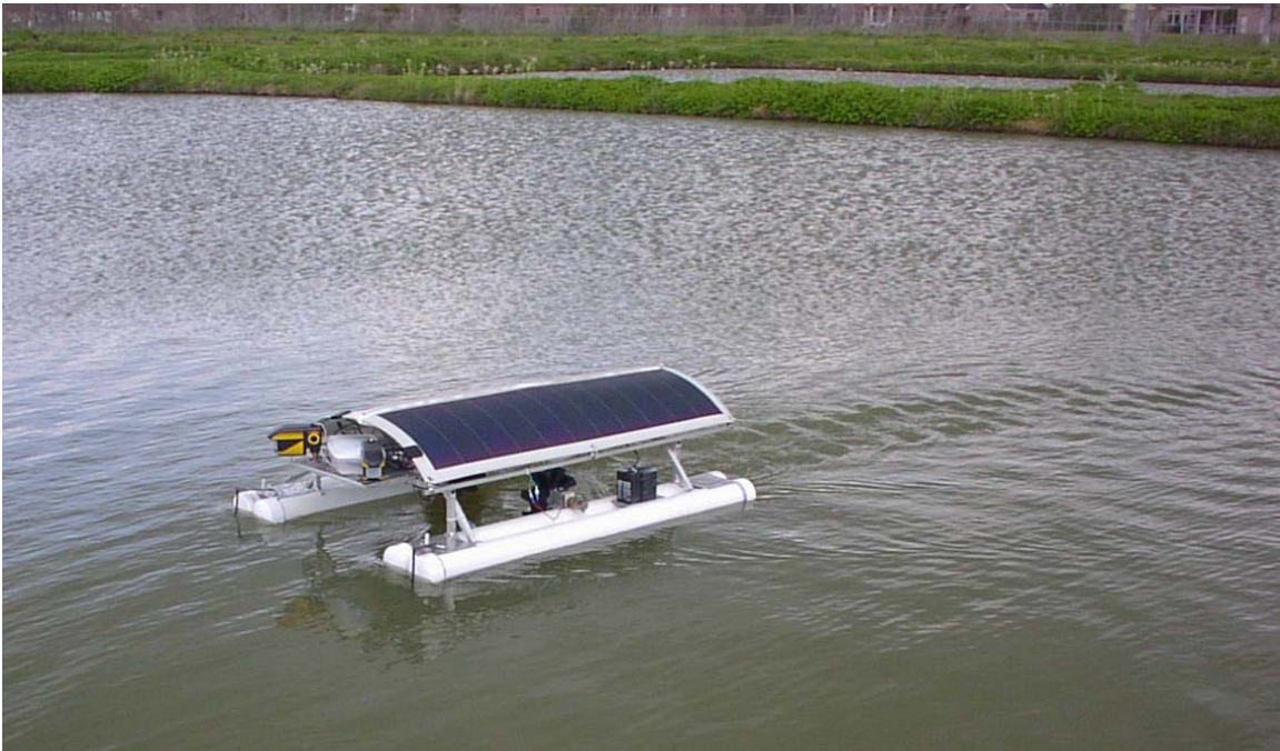
Fig: 2.1. Autonomous boat built by LSU Agricultural Center
