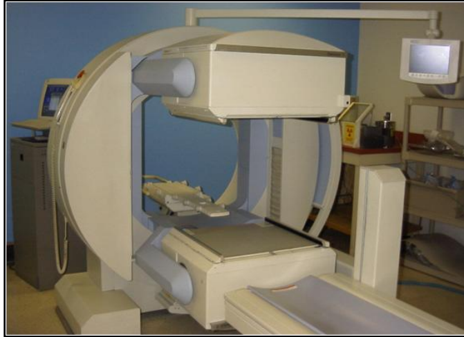
Figure 1. Commercial gamma camera. The two detector heads (above and below) produce a full-body scan with “hot” spots indicating where a radiopharmaceutical has accumulated.
