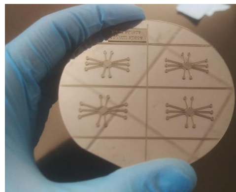
Figure 3.5. Silicon wafer with orthogonal design. Chosen geometry was a 3 mm diamond side length and a 150 \mu\text{m} spacing between outer channels and central diamond.
