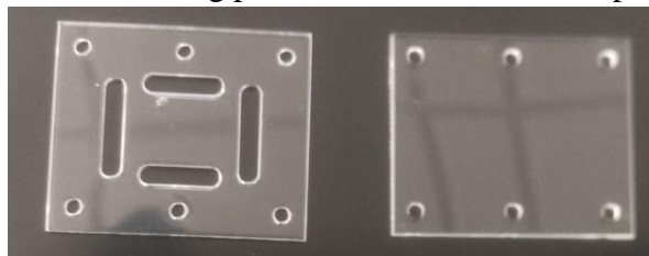
Figure 3.8. Completed orthogonal Plexiglas pieces after being cut out using a laser printer.
