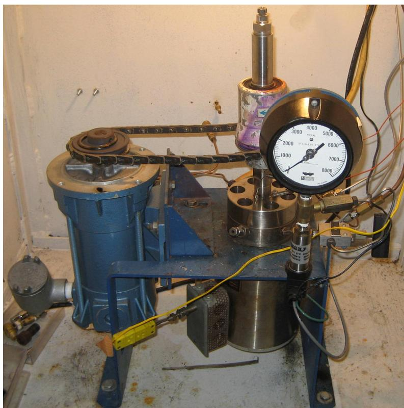
Figure 1.4: Picture of the 300ml HTL Processor at LSU.
