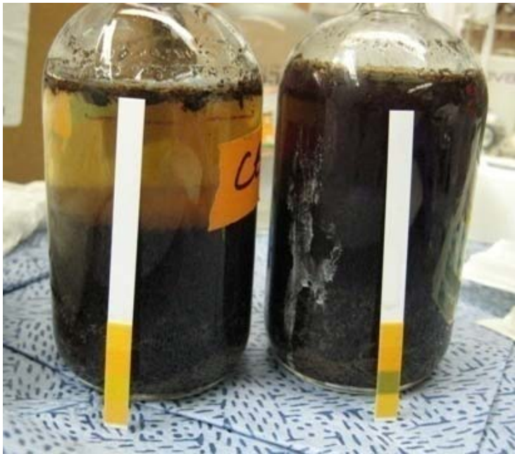
Figure 3.7. Color change in microcosm after pH was neutralized (right) versus acidic microcosm (left).
