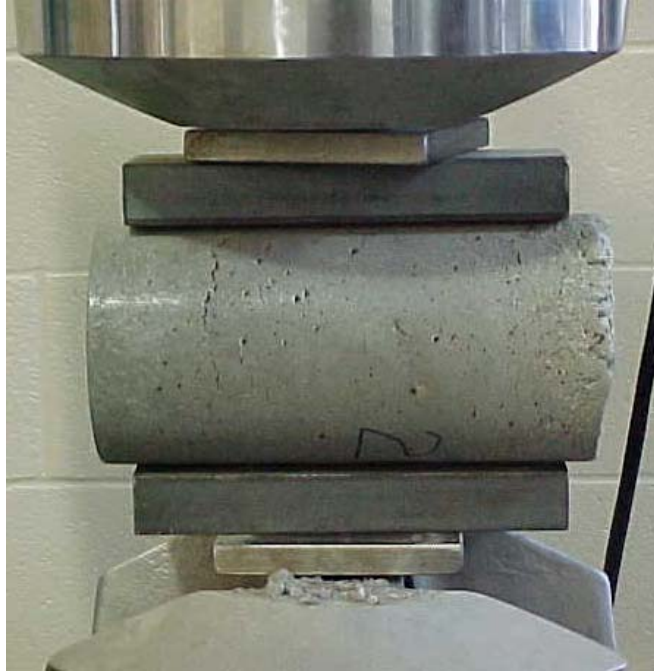
Figure 4: Split tensile strength testing of concrete.
