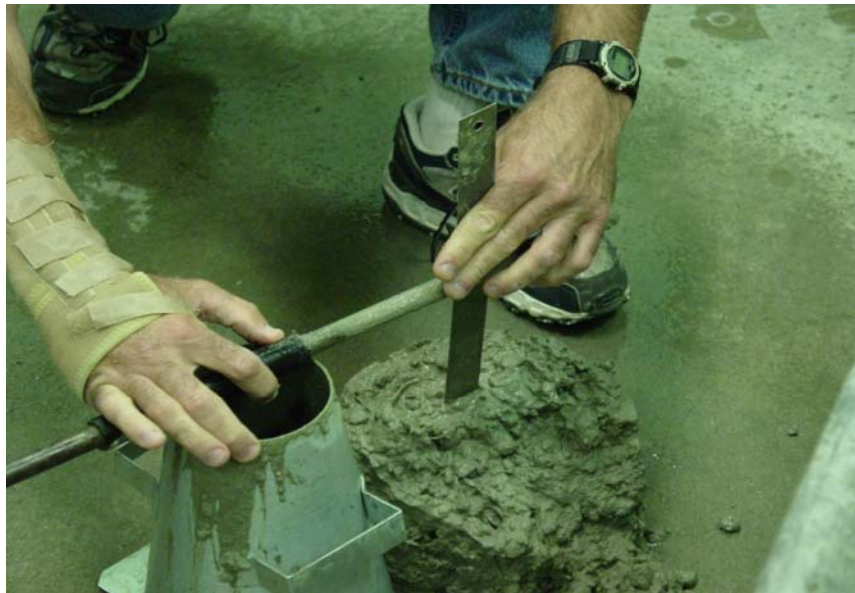
Figure 5: Slump testing concrete
