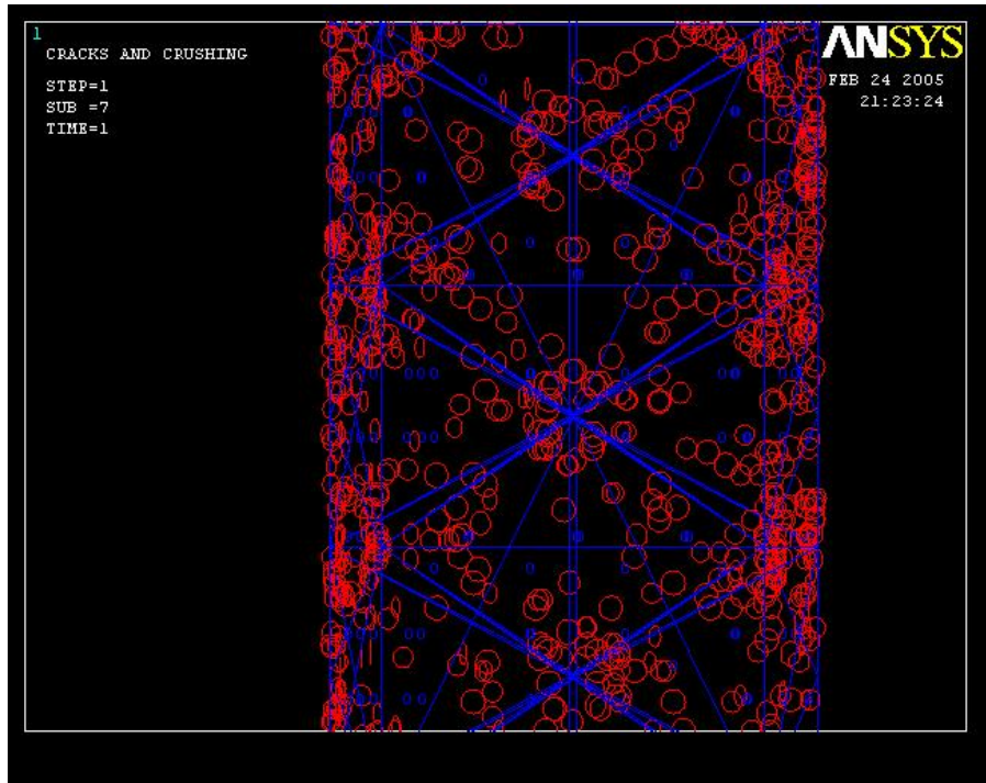
Figure 9: First cracks formed in concrete surrounding fiber on application of load.
