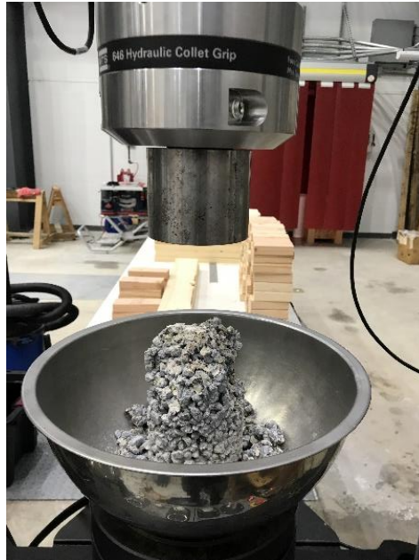
Figure 3. 10.16 cm Diameter x 15.24 cm Tall Curb Sample Crushed.
