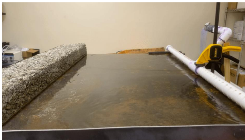
Figure 6. Permeable Curb in Metal Crate.
