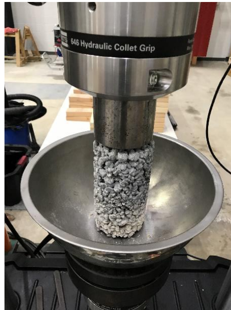
Figure 2. 10.16 cm Diameter x 15.24 cm Tall Curb Sample.
