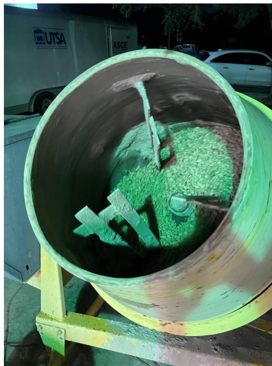
Figure 1. Concrete Mixer for Pouring of Permeable Curb.
