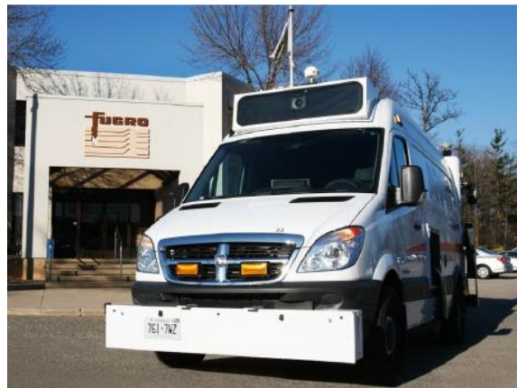
Figure 6. The Automatic Road Analyzer (ARAN) system
