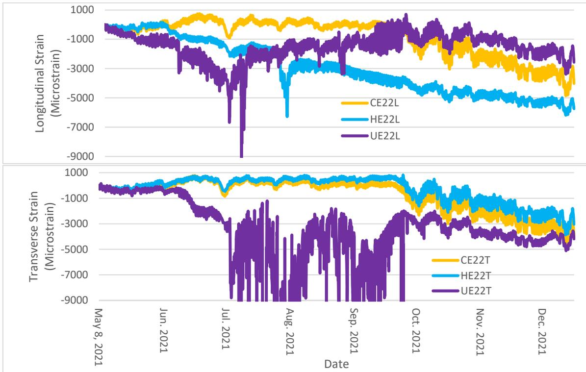
**Figure 110. Longer-term longitudinal and transverse strain in eastbound lane - bay 2 – position 2.**
