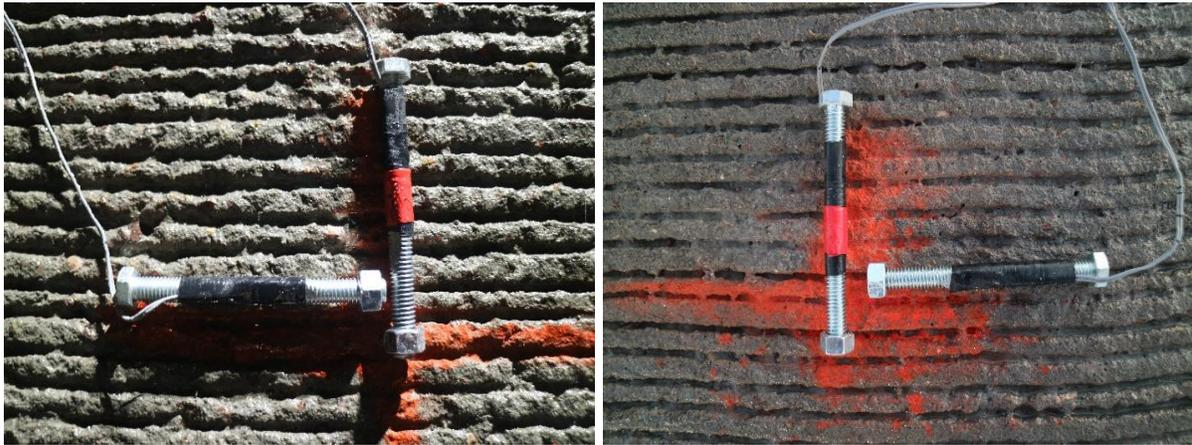
**Figure 30. Embedded sensor installation in UHPC overlay.**
