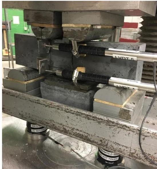
**Figure 20. UHPC prismatic sample at failure during flexural test.**
