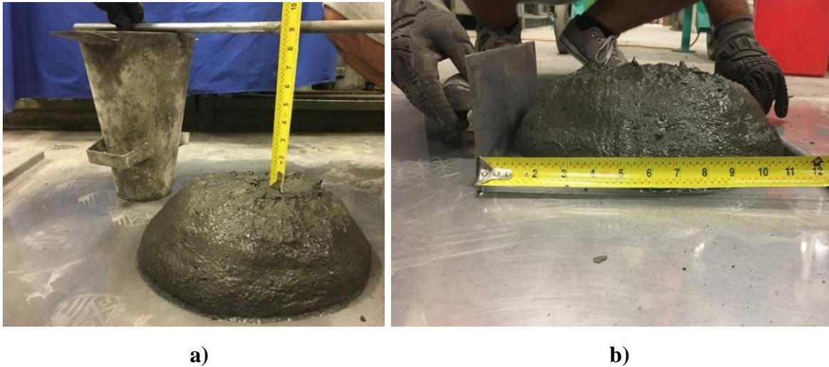
Figure 18. a) Slump and b) spread measurements.
