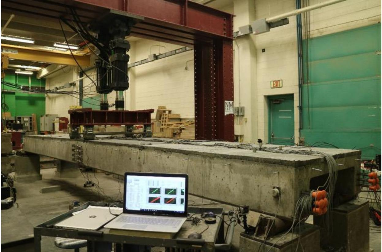
Figure 5. UHPC overlaid girder flexural testing setup (1).
