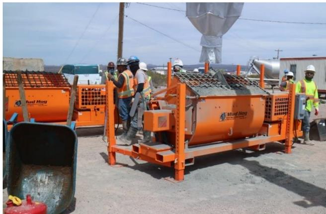
**Figure 14. Horizontal shaft mixers.**
