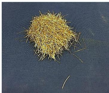
Figure 2. Steel fibers used for UHPC fiber reinforcement.
