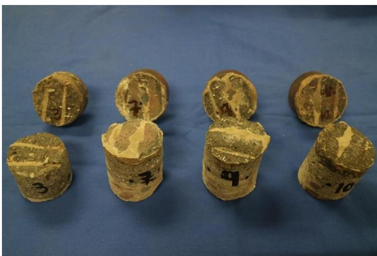
Figure 77. UHPC/epoxy failure.
