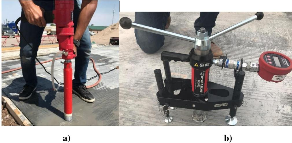
**Figure 21. a) Core drilling and b) pull-off test setup.**
