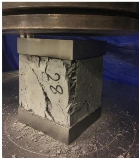
Figure 19. UHPC cube sample at failure under compression test.
