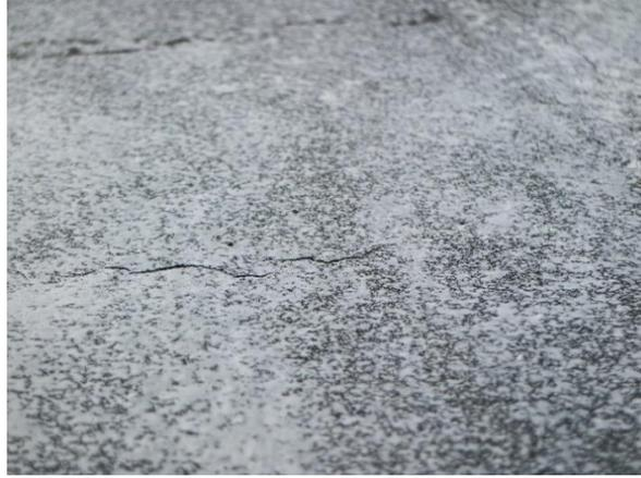
Figure 17. Mock-up placement 4 – UHPC overlay cracking.
