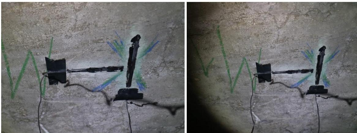
Figure 28. External sensor installation inside box girder cells.
