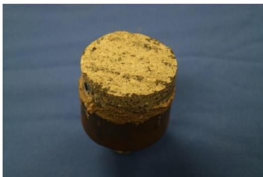
Figure 76. Core sample with substrate that lacks roughness.
