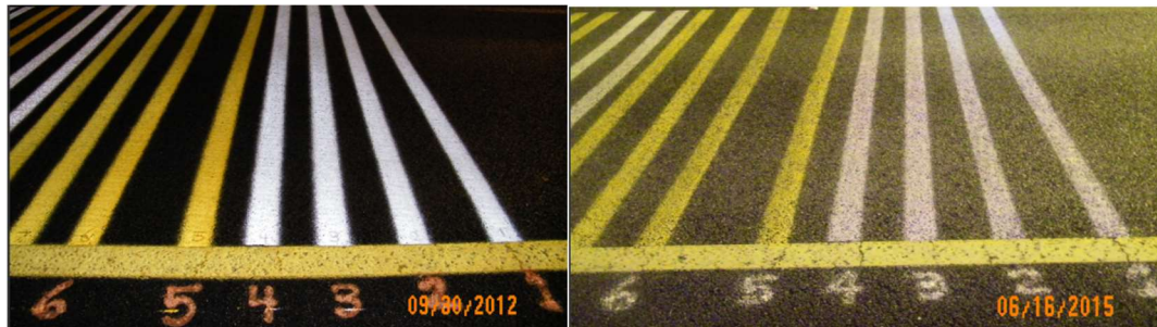
Figure 1 White and yellow paints after installation (left) and after 36 months (right) for one of the waterborne paints applied in Florida
