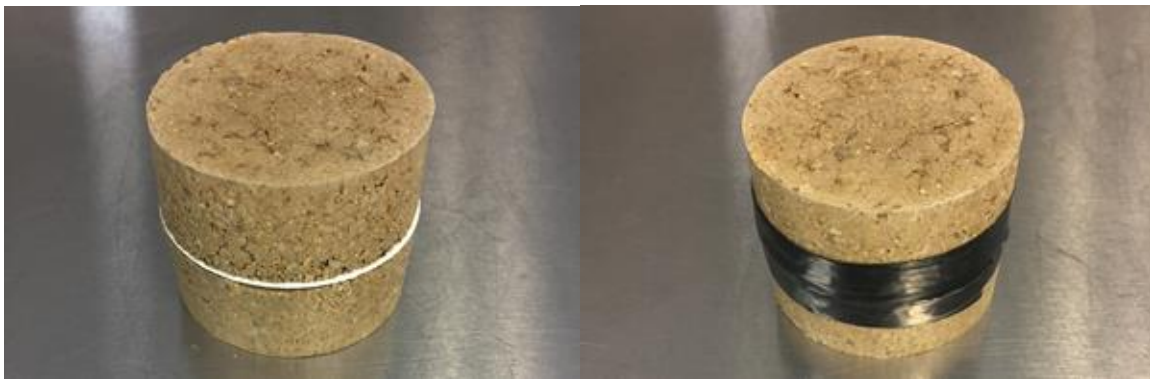
Figure 7. Two stacked soil specimens with a filter paper in-between (left); filter paper sealed with electrical tape
