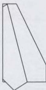
Fold one wing such that the outer edge is brought colinear with the plane's centerline
