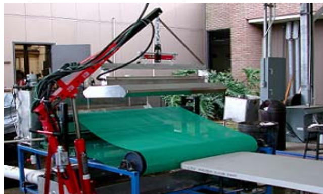
Fig. 16 – The infrared heater placed above the belt
