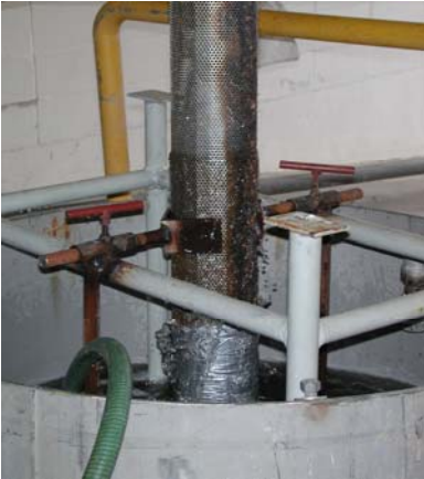
Fig. 7 – The wet cylindrical depither
