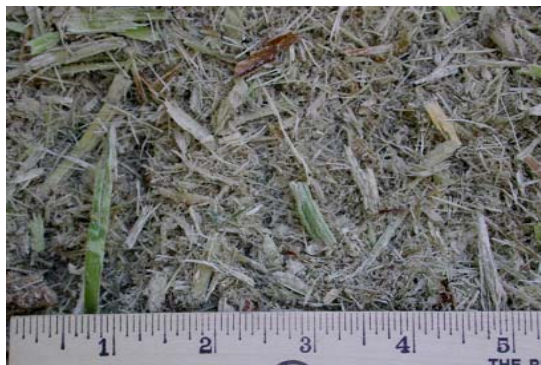
Fig. 2 – Mill run bagasse, South Louisiana Sugars Cooperative, 2005 (scale in inches)
