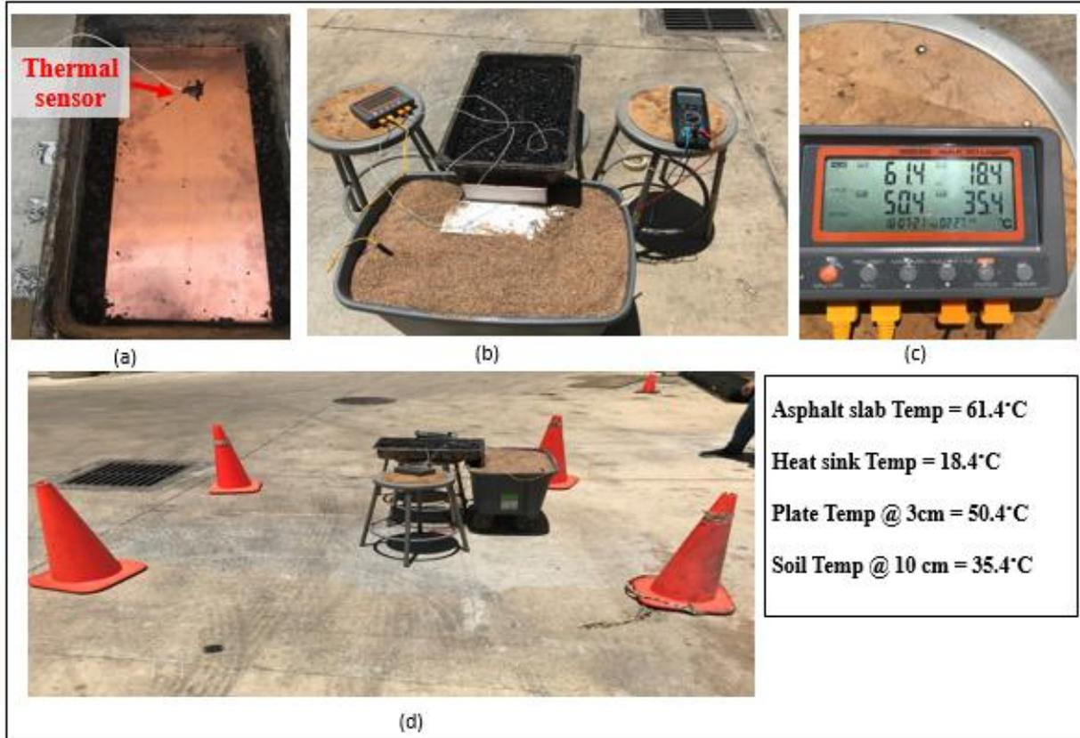
**Figure 20. Field installation and data collection.**
