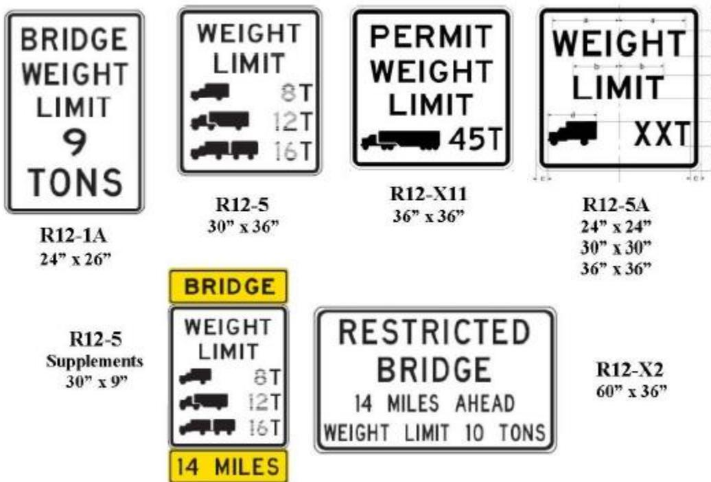
Figure 5. Load Posting Signs (Source: BSIPM by MnDOT)
