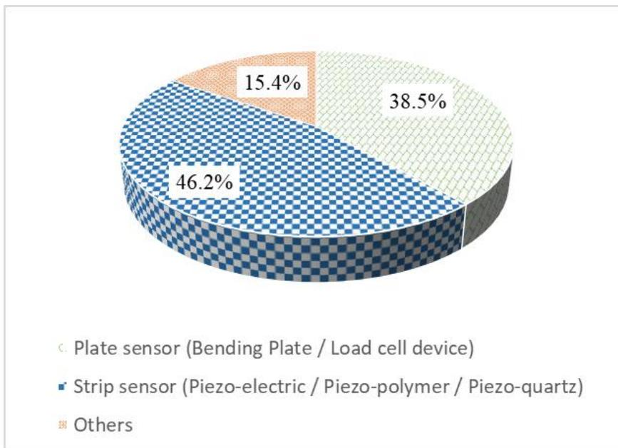
**Figure 43. Sensor Type Used in WIM**
