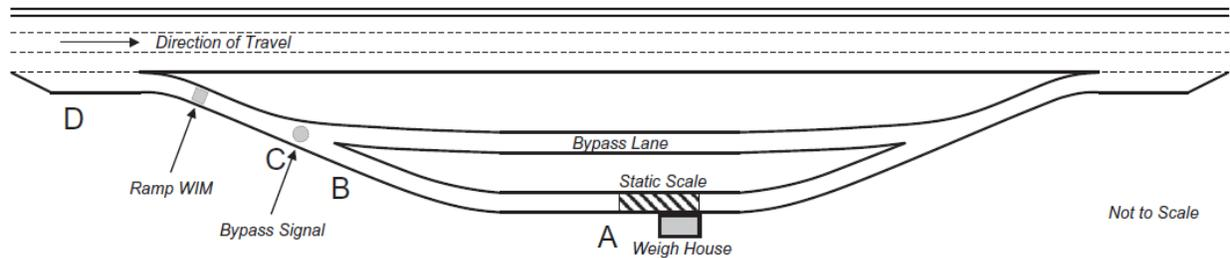
**Figure 21. Concept of Weigh in Motion System (Source: Adaptive weigh-in-motion algorithms for truck weight enforcement)**
