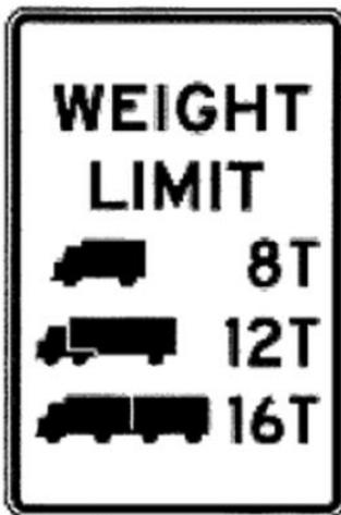
Figure 3. Load Posting Sign for Special Hauling Vehicle (SHV) Load (Source: ADOT Bridge Load Rating Guidelines)
