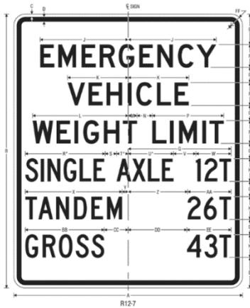
Figure 4. Load Posting Sign for Emergency Vehicle Load (Source: ADOT Bridge Load Rating Guidelines)
