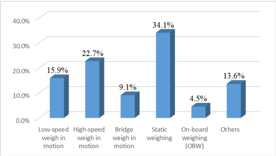
Figure 41. Current Enforcement Technology Used for Bridge Weigh Monitoring in the US
