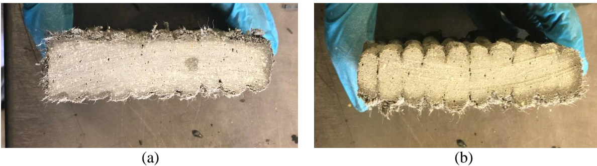
Figure 22. Cross-sections of walls printed for buildability evaluation (left to right) (a) at 0 minutes time gap (b) at 5 minutes time gap
