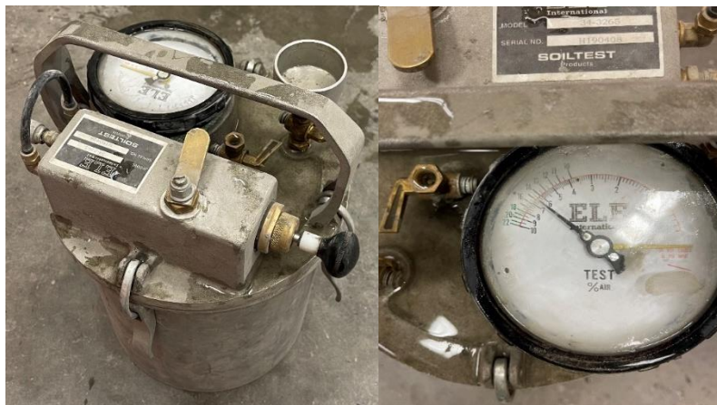
Figure 4. Air content test.
