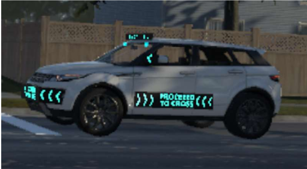
Figure 8. Side-displayed eHMI on driver side door.
