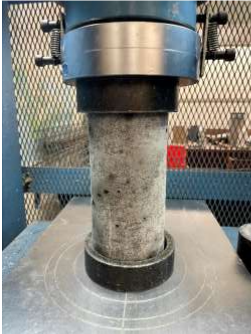
Figure 9. Compression test setup.
