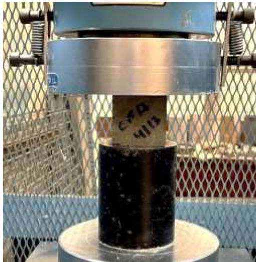
Figure 6. Compressive strength testing setup for 50.8-mm (2-in) mortar cubes.
