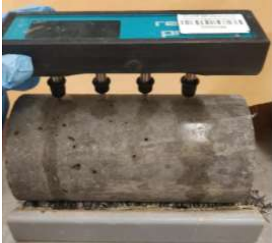
Figure 10. Surface resistivity setup.
