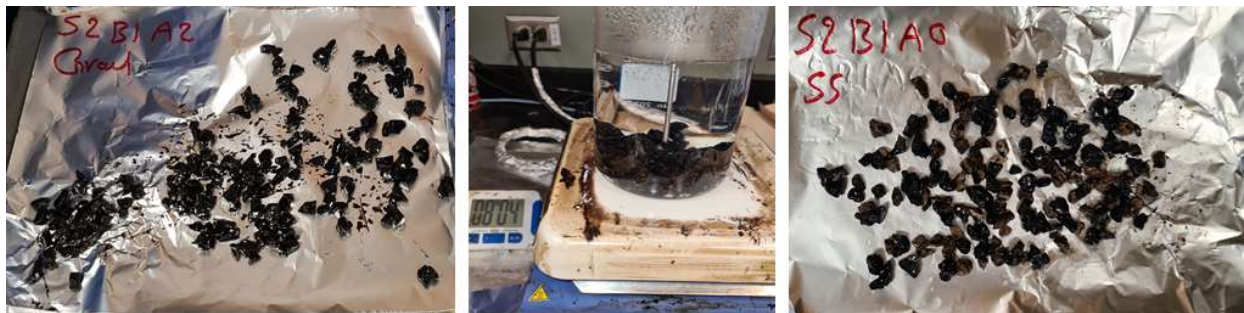
Figure 18: Texas Boiling Test; separating coated aggregates (left), boiling the sample (middle), and air drying after boiling (right).
