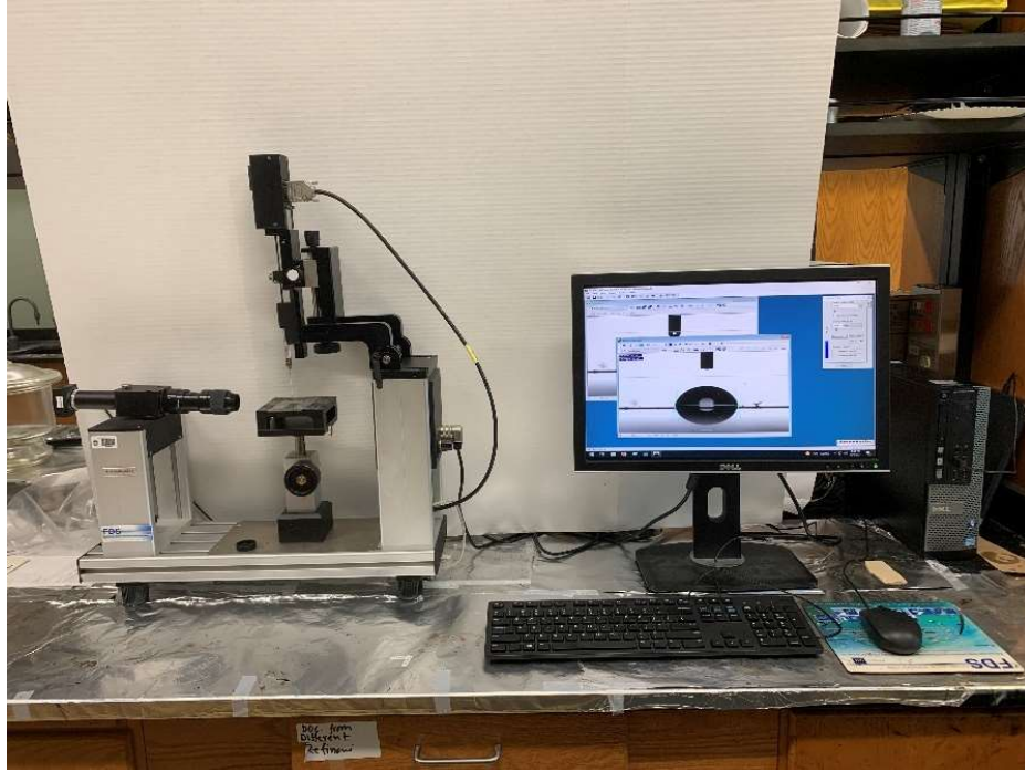
Figure 17: Sessile Drop test set up.
