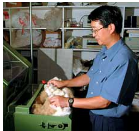
Yan Chen feeds bagasse, a waste product from sugarcane, along with bonding fibers into a universal carding machine at the LSU AgCenter's Textile Processing Laboratory.
