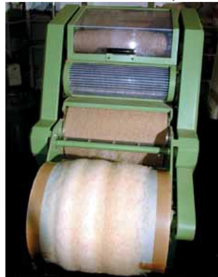
After being cleaned, the bagasse is blended with bonding fibers for forming a fiber web.
