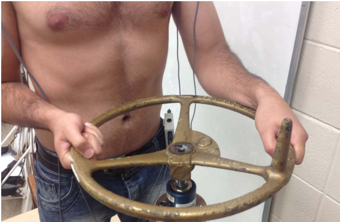
Figure 51: Hand placement locations during maximal isometric torque exertions.
