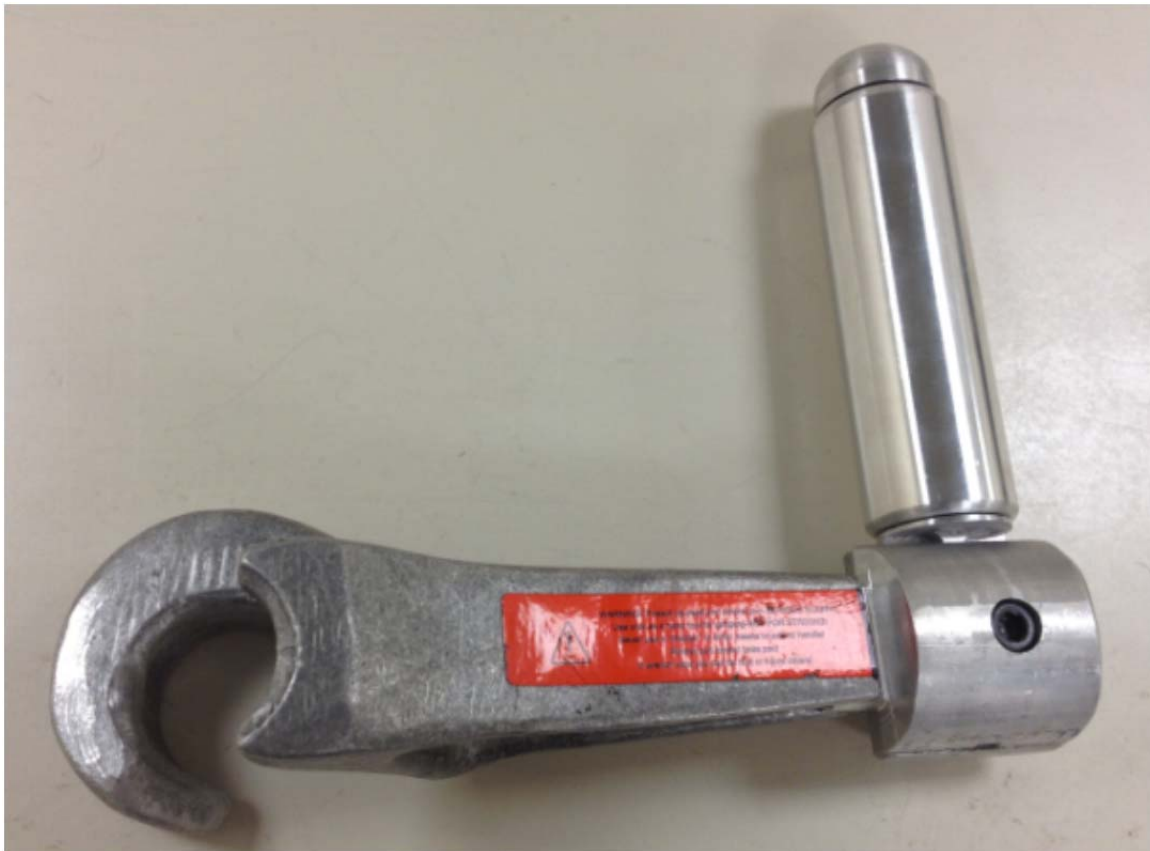
Figure 37: A prototype of the modified wrench that includes a locking joint using an allen screw.
