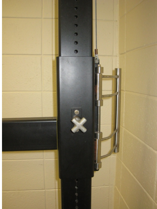
Figure 40: The lever arm can be moved along the vertical post and clamped at any desired height.
