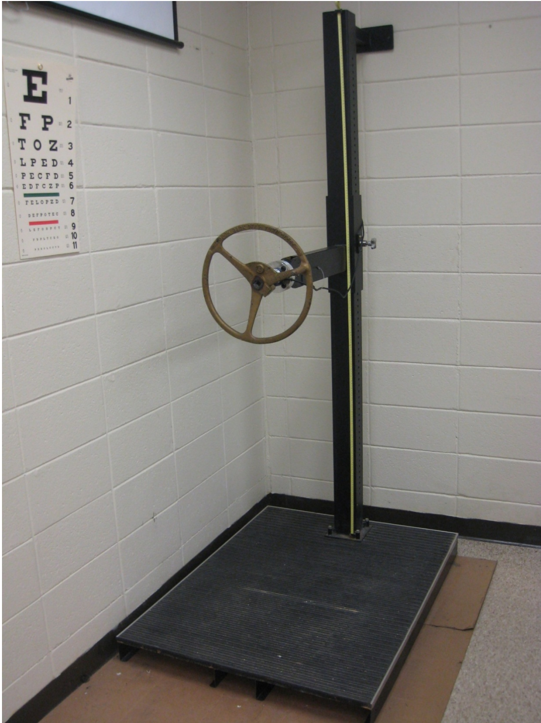
Figure 39: Isometric strength testing equipment (Prototype Design and Fabrication Company, Ann Arbor, MI, USA).
