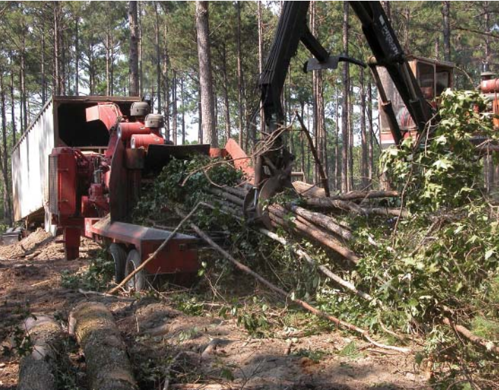
Travis Taylor Logging & Chipping, of Winn Parish, removes understory trees and brush on the Kisatchie National Forest and on private timberlands. Here, the loader (right) feeds whole trees into the chipper (left), which blows the chips into the truck behind it. The chips are utilized for paper and energy at a nearby paper mill.
