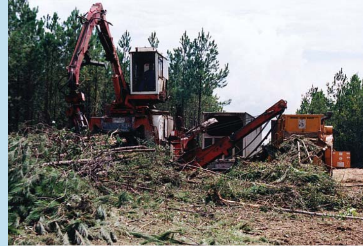
Like overcrowded garden plants, young pine trees need to be thinned out. Several logging contractors in Louisiana specialize in bringing whole trees out of the woods, chipping the whole trees into 2-inch pieces and sending the chips to paper mills. The stems make good quality chips for paper, while the limbs are ground into boiler fuel for cogeneration.
